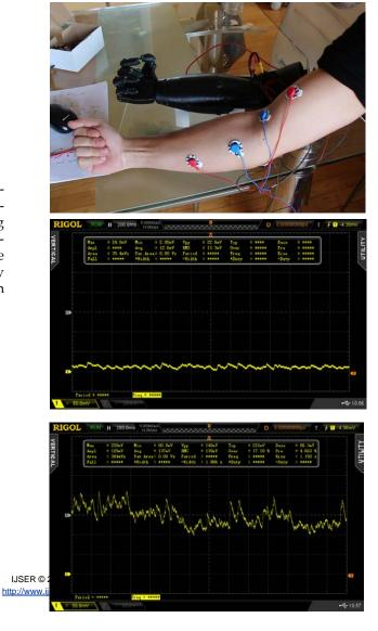
As illustrated below the sampled points used for servo control are constantly shifting up and down. A smooth signal is desired which means some filtering should be done to these EMG outputs to improve control characteristics. Increasing the time between ADC samples and servo updates slows down the shaking of the fingers but does not fix the problem.
